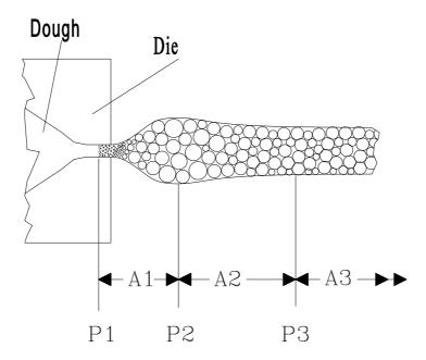
The expansion can be seen as a phenomena limited by time, starting from the point of time, where the still existing pressure has just sunk down to such a level that water, which is present in the dough in an overheated state, begins to evaporate.
